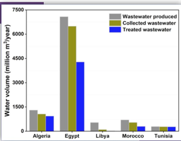
Figure 10 - State of Wastewater collection and purification
